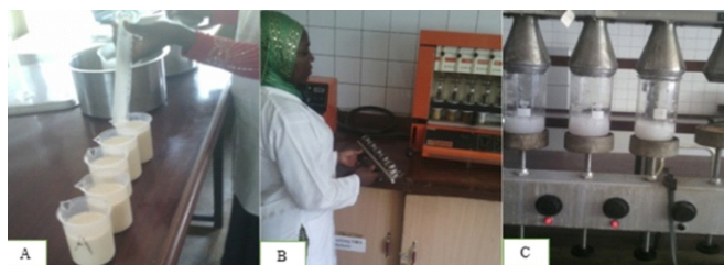
Figure 2: Formulating different blends of maize based-soy milk ( A ), loading samples into the Soxhlet machine for crude fat determination ( B ), and determination of dietary fibre content in the products ( C ).
